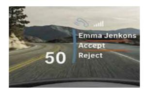
The Head-Up Display projects a multi-color image that seems to float beyond the windshield, just below your line of vision. The onscreen data is projected thanks to HARMAN technology rooted in the infotainment system. It allows you to monitor preferred travel information, such as current speed, BMW Navigation system directional arrows and posted speed limit, as well as check control data and more—without taking your eyes off the road.
