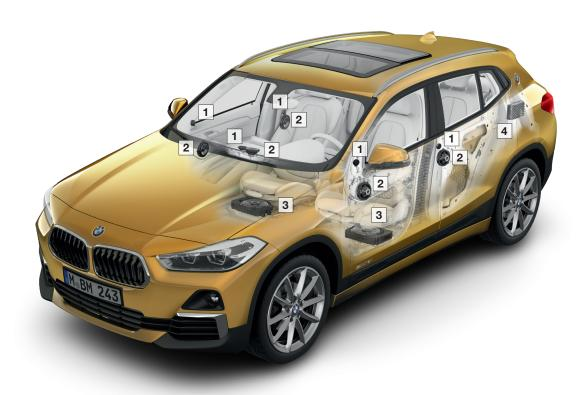
5 x 26 mm metal-matrix dome tweeters, dashboard, front, and rear side
