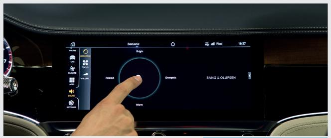
**Sound field.** Moving the white marker on the fixed x- & y-coordinates creates the unique sound desired.
